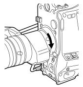
4 Press the cable into the cable clamp and connect it to the LENS connector.
